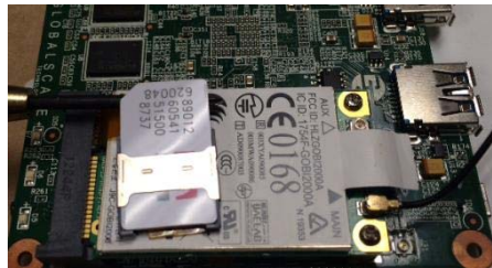
Figure 6. Example of a cellular enabled skimmer
