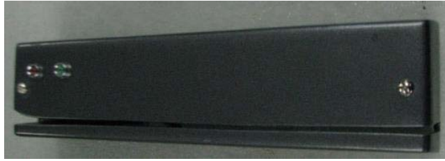
Figure 5. Example of a custom skimmer (door)
