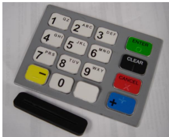
Figure 14. Example of keypad overlay
