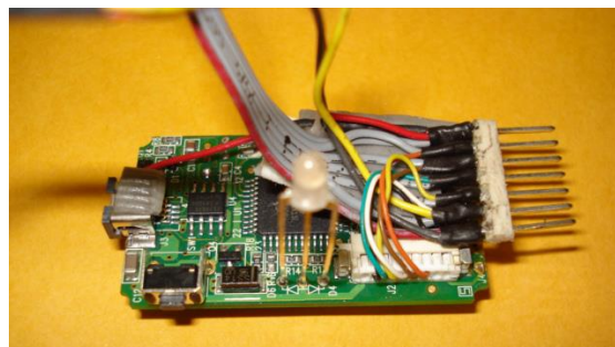
Figure 2. Example of an altered hand-held skimmer
