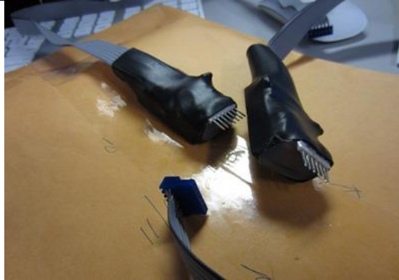
Figure 15. Example of an inline skimmer
