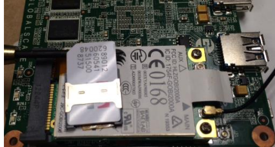
Figure 6. Example of a cellular-enabled skimmer
