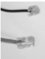
RJ45 LAN Cable & RJ11 Phone Cable
